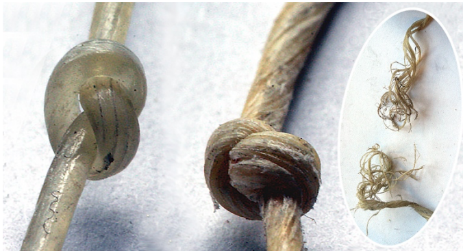
Figure 5: A comparison of good quality natural gut (left), and poor quality natural gut (right). Inset: the failed poor-quality line
